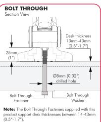
M8 bolts can be used to suit desk thicknesses outside this range. Bolt length=desk thickness+25mm (1").
