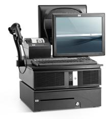
HP rp5800 POS System shown with Integration Assembly (4 parts, each sold separately) and assorted peripherals, including: barcode scanner and mount, cash drawer, printer, keyboard with MSR, 15" diagonal employee-facing touch display, and a 15" diagonal customer facing display (left) or customer facing 2-line display (right).
