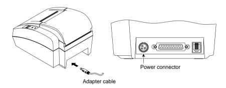
NOTE: To remove the DC cable connector, make sure that the power supply's power cord is unplugged; then grasp the connector at the arrow and pull it straight out.
