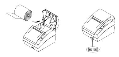
NOTE: When closing the cover, press the center of printer cover firmlay to prevent Paper miss-loading.
