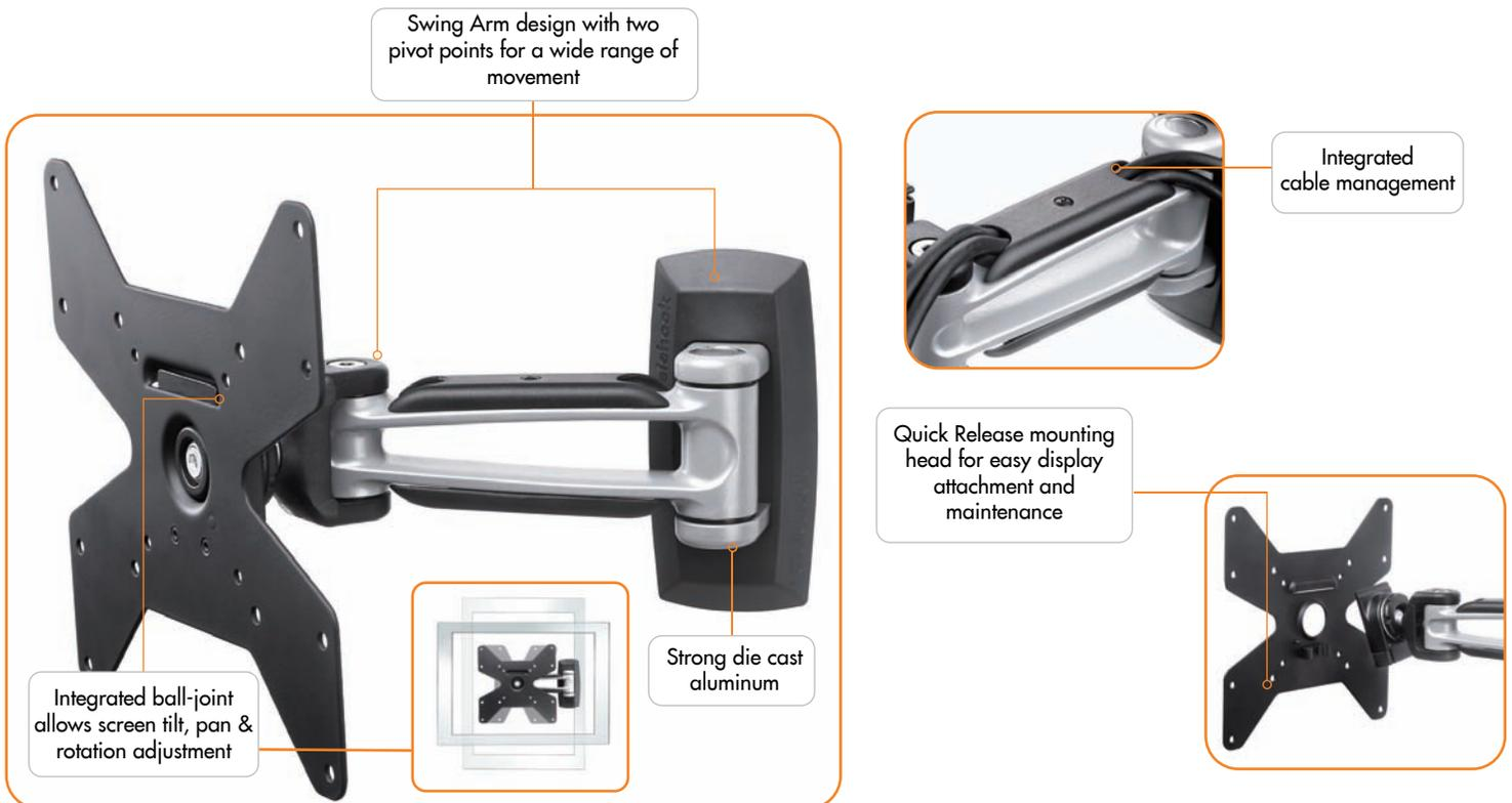
\* Supports 75x75, 100x100, 200x100 & 200mmx200mm VESA hole patterns. Also supports 200x300, 200x400, 300x200, 300x300, 300x400, 400x200, 400x300 & 400mmx400mm via optional adaptor accessory
