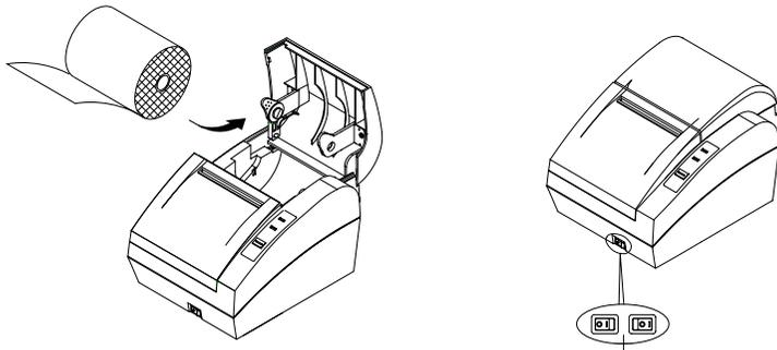
**NOTE :** When closing the cover, press the center of printer cover firmly to prevent Paper miss-loading.
