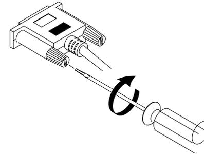
3. Attach the other end of the cable to the computer.
