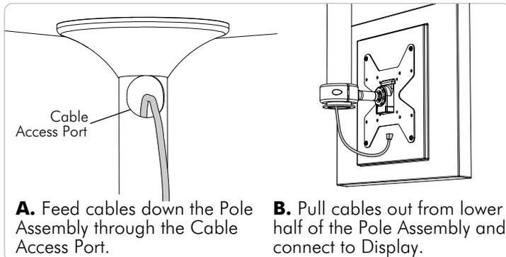
**A.** Feed cables down the Pole Assembly through the Cable Access Port.
