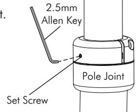
**D.** If necessary, centralise the Pole Joint by tightening the Set Screws (x2) to suit.
