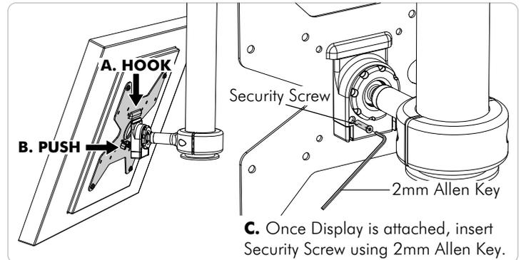
**C.** Once Display is attached, insert Security Screw using 2mm Allen Key.
