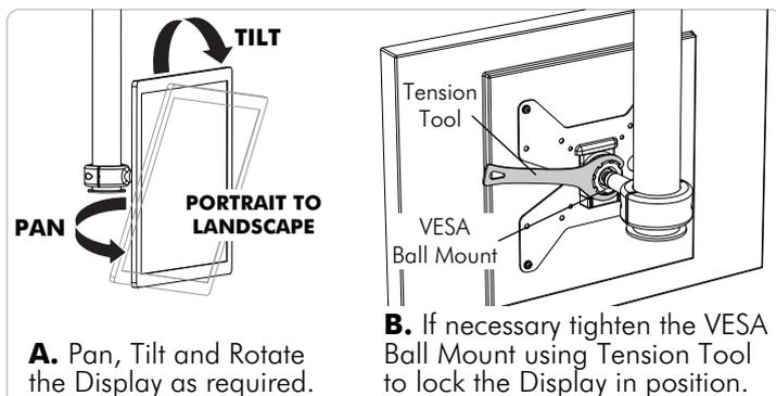
**A.** Pan, Tilt and Rotate the Display as required.
