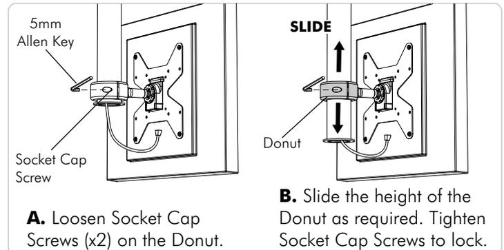
**A.** Loosen Socket Cap Screws (x2) on the Donut.
