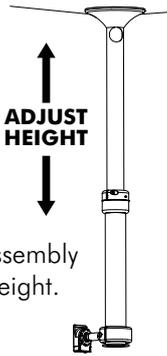
**C.** Tighten the Socket Cap Screws (x2) to set the height.
