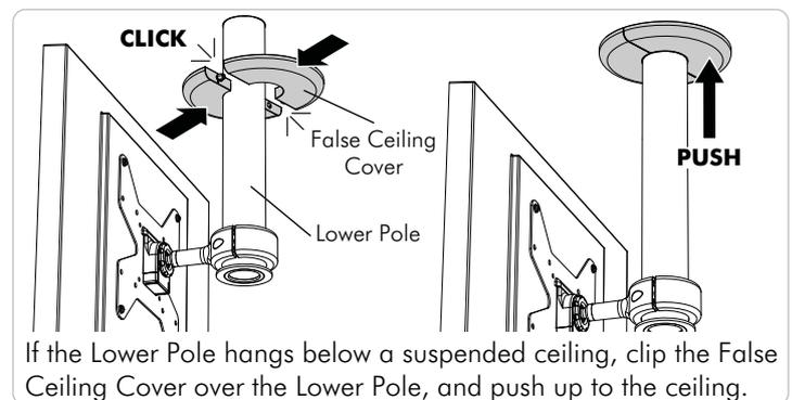
If the Lower Pole hangs below a suspended ceiling, clip the False Ceiling Cover over the Lower Pole, and push up to the ceiling.
